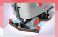
The squeegee can follow all machine movements precisely thus ensuring perfect drying without any mark being left behind. The operator can easily adjust the squeegee tilt by simply turning the two screw knobs. The rubber bars can beused on all 4 edges and can be easily removed and replaced thanks to the specially designed clamps
