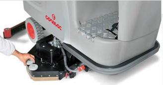
The sweeping-scrubbing unit has been designed to offer a solution to more demandino cleaning tasks and it is suitable for more stubborn dirt. It is in fact provided with a cylindrical brush system which, not only scrubs, but also picks up solid dirt (cigarette butts, wood shavings, small metal residues, etc.) and conveys it into a special hopper which can be easily removed for emptying
