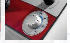
It is possible to choose 3 different working speeds and brush pressure levels to adjust the machine to any conditions.
