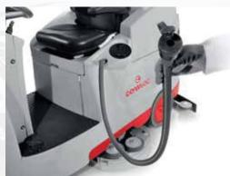
The length of the hose for solution tank filling (optional) allows to directly and comfortably reach a water tap.
