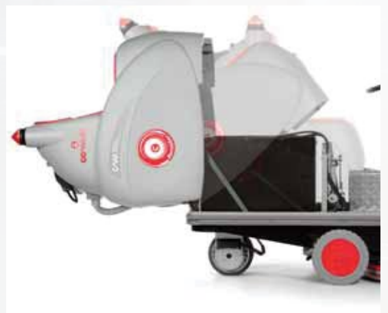
Wide bonnet opening for best access to the battery compartment
