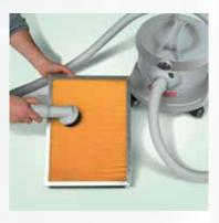
It is important to clean the panel filter with a vacuum cleaner after each cleaning task in order to guarantee perfect machine performance
