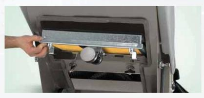
The panel filter can be easily replaced without the help of any tools. The electric filter shaker, on request, ensures an automatic cleaning of the filter.
