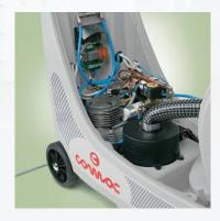
The internal compressor ensures optimal foam formation. The two-stage suction motor removes rapidly and thoroughly the product from the fabric that has been treated
