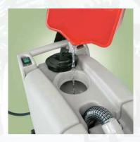
The 20 litre capacity of the solution tank ensures very long operating autonomy thanks to the usual low consumption rate of foam systems
